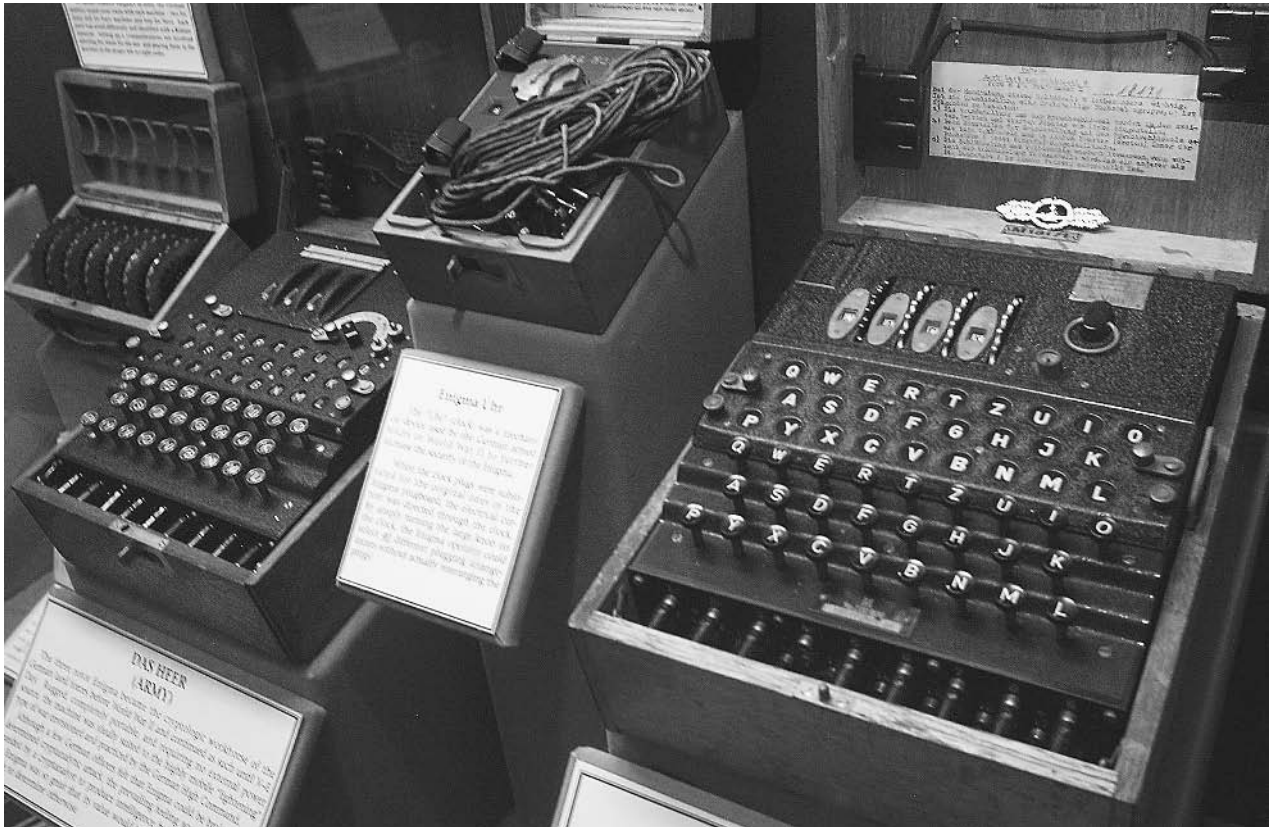
A four-rotor Enigma machine, right, which was used by the crews of German U-boats in World War II to send coded messages. AP/WIDE WORLD PHOTOS.
