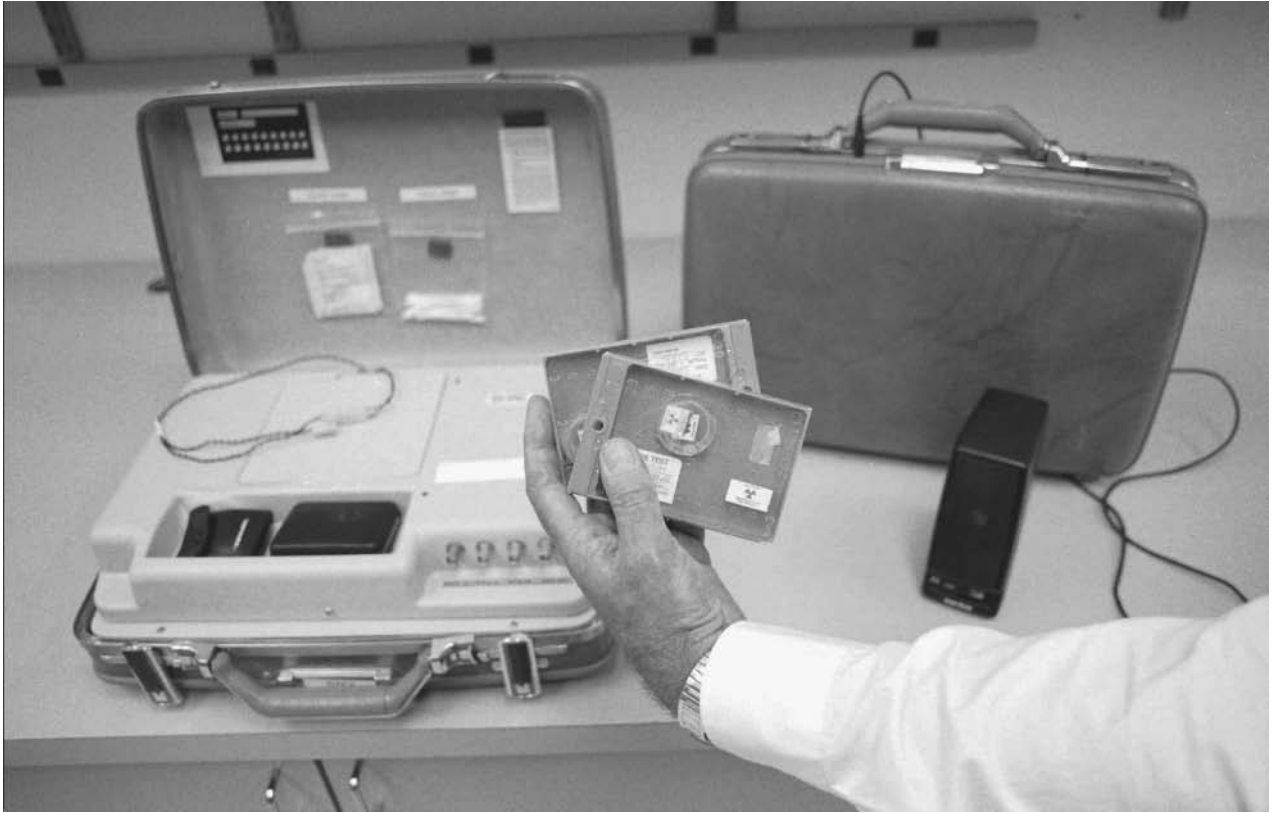
A Nuclear Emergency Search Team (NEST) member shows portable sensing equipment used to detect radioactive sources. The briefcase design allows NEST members to carry the sensing device undetected in crowded environments. AP/WIDE WORLD PHOTOS.
