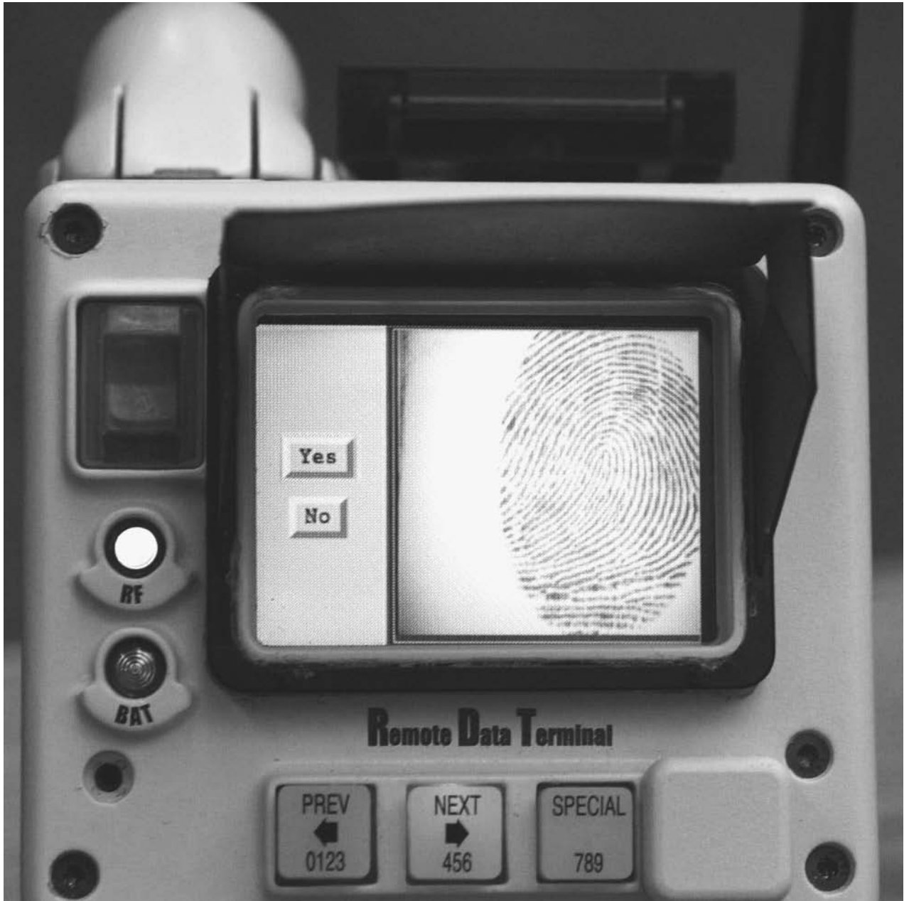
A fingerprint is seen on the back of a wireless device called an "IBIS." It can record a fingerprint in the field, then send the fingerprint via a wireless connection to be checked against a database. AP/WIDE WORLD PHOTOS.
