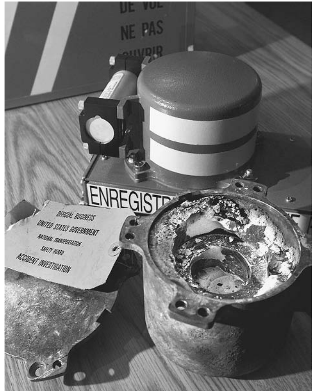
The charred casing of the flight data recorder recovered from the crash of American Airlines flight 587 is displayed at the National Transportation Safety Board in 2001, along with a normal, undamaged flight recorder (at rear). AP/WIDE WORLD PHOTOS.
