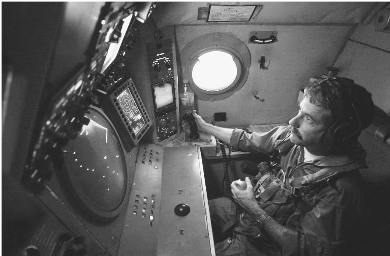
A U.S. Navy aviation systems warfare operator searches for and tracks surface contacts using radar and the Infrared Detection System of his P-3 Orion patrol aircraft during a routine flight in support of Operation Enduring Freedom in October 2001. AP/WIDE WORLD PHOTOS.
