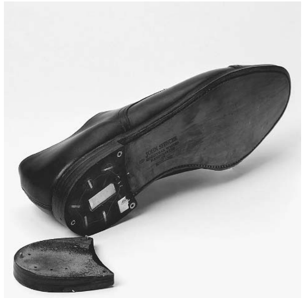
A shoe with an imbedded heel transmitter produced by the KGB during the Cold War to monitor secret conversations. ©AFP/CORBIS.
