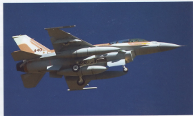
Right: Aircraft number 00-1020, tail number 440, approaching landing after a test flight. The payload consists of two 370 gallon underwing and a 300 gallon centerline external fuel tanks.
