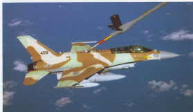
Left: The second F-16I of the first pair delivered was aircraft number 00-1006, tail number 408, during air refueling from a USAF KC-135 on-route to Israel. Noteworthy is the USAF Marking applied only to the right wing, while the IAF markings are covered.
